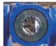
T-axis hollow arm: 50 mm dia.
