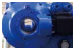
R-axis hollow arm: 50 mm dia.
